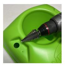
A 7/8" drill bit is needed. Ver-tech recommends a Step Bit for seamless customization.
